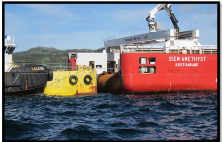
The anchor handling tug supply vessel SIEM Amethyst working in tandem with the Kaliutik to ensure accurate placement of a mooring component at the deep water site of Bull Arm.
